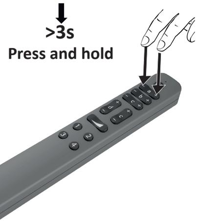
The successful start is confirmed by a fast flashing of the red indicator LED. If the connection is successful, the red LED flashes 6 times. The successful connection is also confirmed by the flashing of the connected LED light
