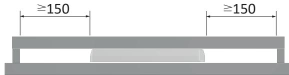
LED ballast - This device should be accessible for maintenance.
